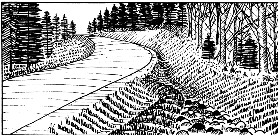
A turnout directs runoff from a ditch into a vegetated buffer area.
